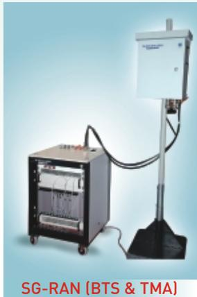
Radio Access Network (RAN), comprises TRAU, BSC and BTS. The SG-RAN solution permits sharing of the RAN by multiple operators / service providers, thereby helping in reducing the CAPEX and OPEX. The shared
